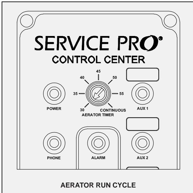
4. Close the control center cover and secure it with a tamper evident seal.
